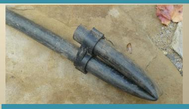
Tip: duck tape or wire to hold hose folded back works just fine
